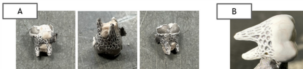
Ceramic tooth after infiltration: A - first trial; B - next attempts
