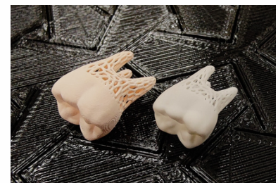
Printed results AES-11C/HSA-0.2 in 20µm layers; A - before and B - after sintering
